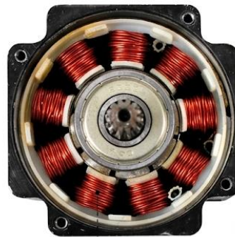
Pure copper motor winding
